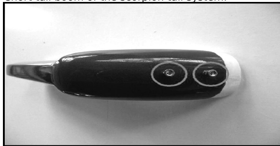
Drill two 1.5mm holes onto the Tail Cover as shown above. Then assemble two Linkage Regulators to these holes.
